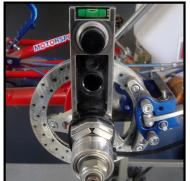
These units will fit any diameter up to 60mm, for non magnetic spindles simply use a cable tie or similar to attach the units
