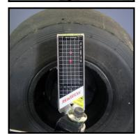
The lnox can be checked for accuracy by recording your settings and then swapping the units left to right and you should see the same settings (toe in/out will be back to front).
