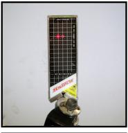
You are now ready to begin adjustment of toe and camber. The laser dot in the center of the grid is the beam shining out at the opposing unit. Readings are then taken from the unit opposite to the stub axle being adjusted.
