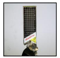
The Inox uses a magnetized Vee Block to locate onto the spindles, therefore the spindles must be clean and free from rust, especially make sure that no metallic debris is stuck to the Vee.
